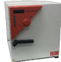
Drying & heating chamber
