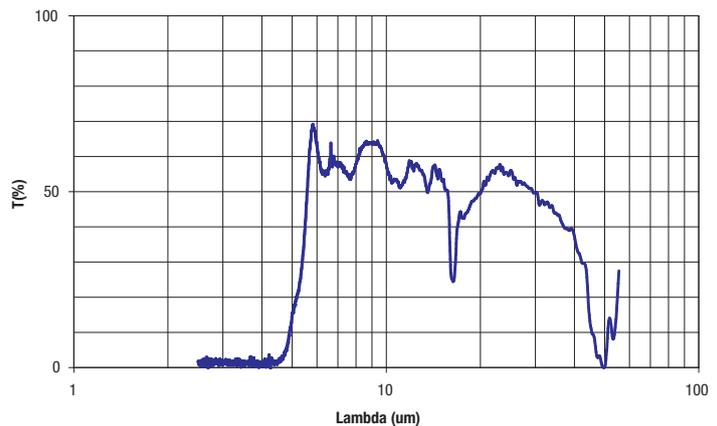
Fig. 2: Transmission of the silicon window.
