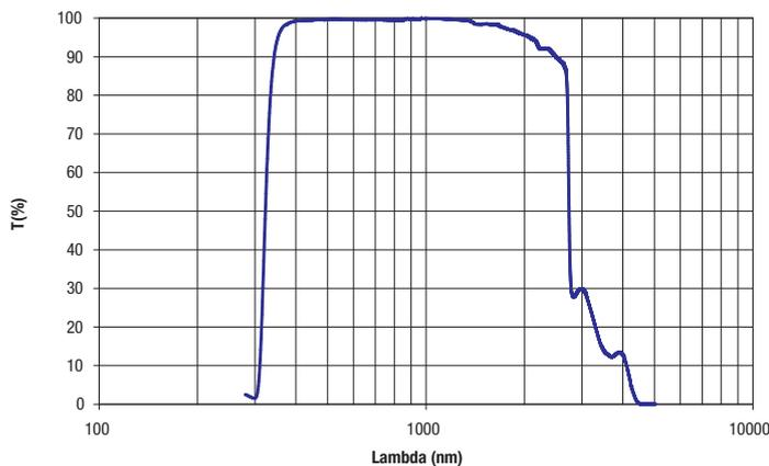
Fig. 1: Relative spectral response of the Delta OHM pyranometers.
